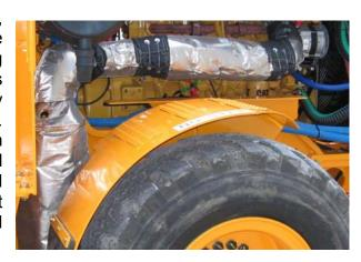
With standard insulation blankets there is a possibility that oils and hydraulic fluids can seep into the underside of the blanket through the mesh inner-liner and lodge in the insulation matt. A build up of oil in the insulation poses a significant danger of spontaneous combustion. A novel solution to this problem had to be found to meet the high safety standards maintained in mines.
